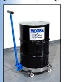
The Clamp+GO™ can be used with round drum dollies of various sizes. Move the quickpin to adjust for 2", 2.5" or 3" (5.08, 6.35 or 7.62 cm) tall dolly sidewall. Clamp+GO™ works with all Morse round drum dollies, and with many
